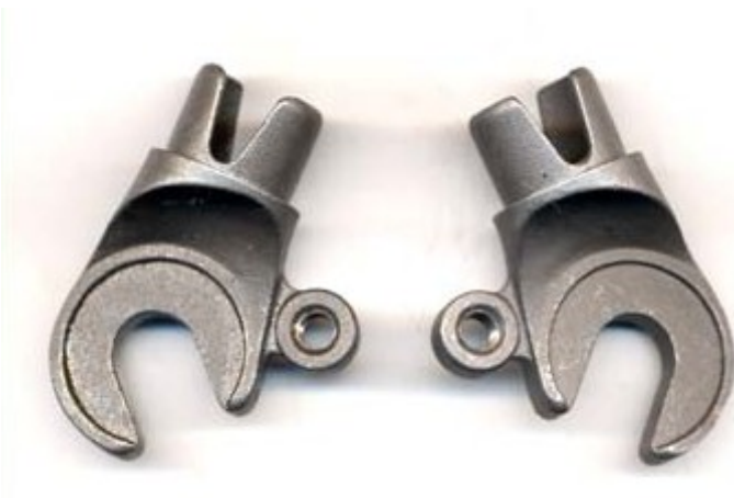
This kind of dropout with overhang above the axle can be problematic for axle mount racks, but OK with a little file work.
